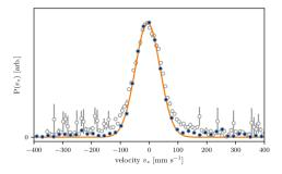
Figure 1: Interferometric measurement of a velocity distribution (filled circles) to which a Gaussian is fitted (solid line) corresponding to a temperature of  $17\mu K$ . Doppler Raman spectroscopy data are also shown (empty circles), revealing differences in the wings.
