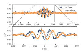
Figure 2: Quadrature interferometer signal measured as a function of  $\tau$ , the temporal asymmetry introduced to the pulse sequence.
